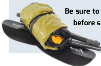
**Be sure to completely dry the TubeBags (including the inside pockets) before storing the boat.**
