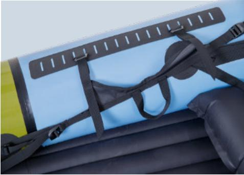
The mat and the boat should now form one unit, the bottom is clearly profiled.
