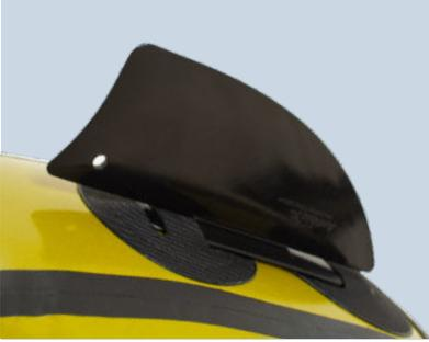
A fin mount is fitted as standard (except Anfibio Nano SL/RTC). It consists of two tabs under the stern of the boat. The optional fin can be easily mounted or dismounted.
